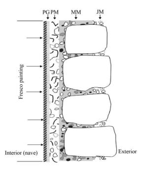
**Fig. 12.** Schematic representation of the distinct layers recognized in the external walls. PG – painting ground, PM – plastering mortar, MM – masonry mortar, JM – joint mortar.
