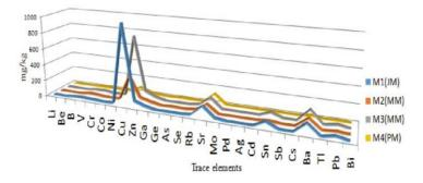
Fig. 14. Concentrations of the trace elements in the studied mortars.
