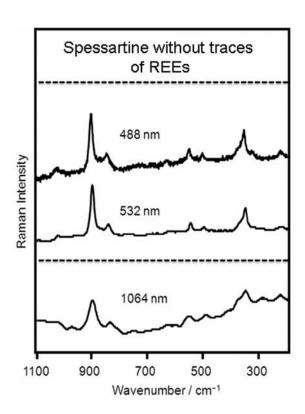
**Fig. 1**. Raman spectra of spessartine obtained by visible (488 and 532 nm) and near-infrared (1064 nm) excitation. The lack of additional bands in the latter spectrum serves to confirm the presence of a very low content of REEs (see Table 1 for details).
