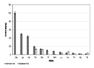
**Fig. 3**. The content of REEs in the studied almandine and spessartine sample determined by  $k_0$ -instrumental neutron activation analysis (error bars are given for k=1, see Table 1 for details).
