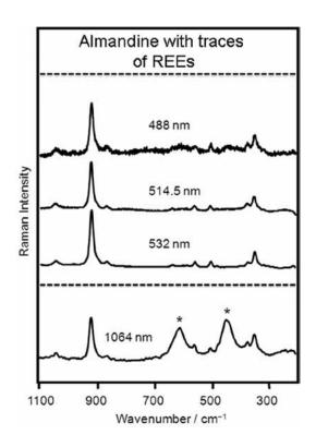
**Fig. 2.** Raman spectra of almandine obtained by visible (488, 514.5, 532 nm) and near-infrared (1064 nm) excitation. The observed additional bands in the latter spectrum (marked by asterisks) are laser-induced fluorescence bands arising from the substantial content of REEs in the sample studied (see Table 1 for details).
