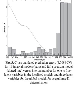
Dotted line is RMSECV (3 LV's) for global model / Italic numbers are optimal LVs in interval model
