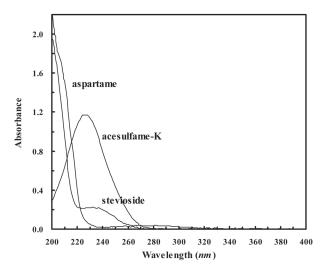
**Fig. 1.** The ultraviolet absorption spectra of pure acesulfame-K, aspartame and stevioside in water. The concentration of acesulfame-K, aspartame and stevioside are 21.28, 48.74 and  $209.0 \ \mu g \cdot m l^{-1}$ , respectively.
