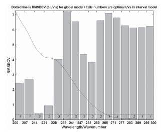
Fig. 5. RMSECV for 16 interval models (bars) and full-spectrum model (line) versus interval number for one to three latent variables in the localized models and three latent variables for the global model, for aspartame determination
