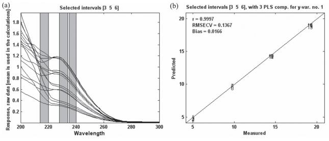
**Fig. 4**. Spectral regions selected to build the models and results: (a) siPLS model by combination of subintervals 3, 5 and 6 for quantification; (b) acesulfame-K content (μg·ml<sup>-1</sup>) vs. the predicted values by cross-validation for the siPLS model with 3 LVs
