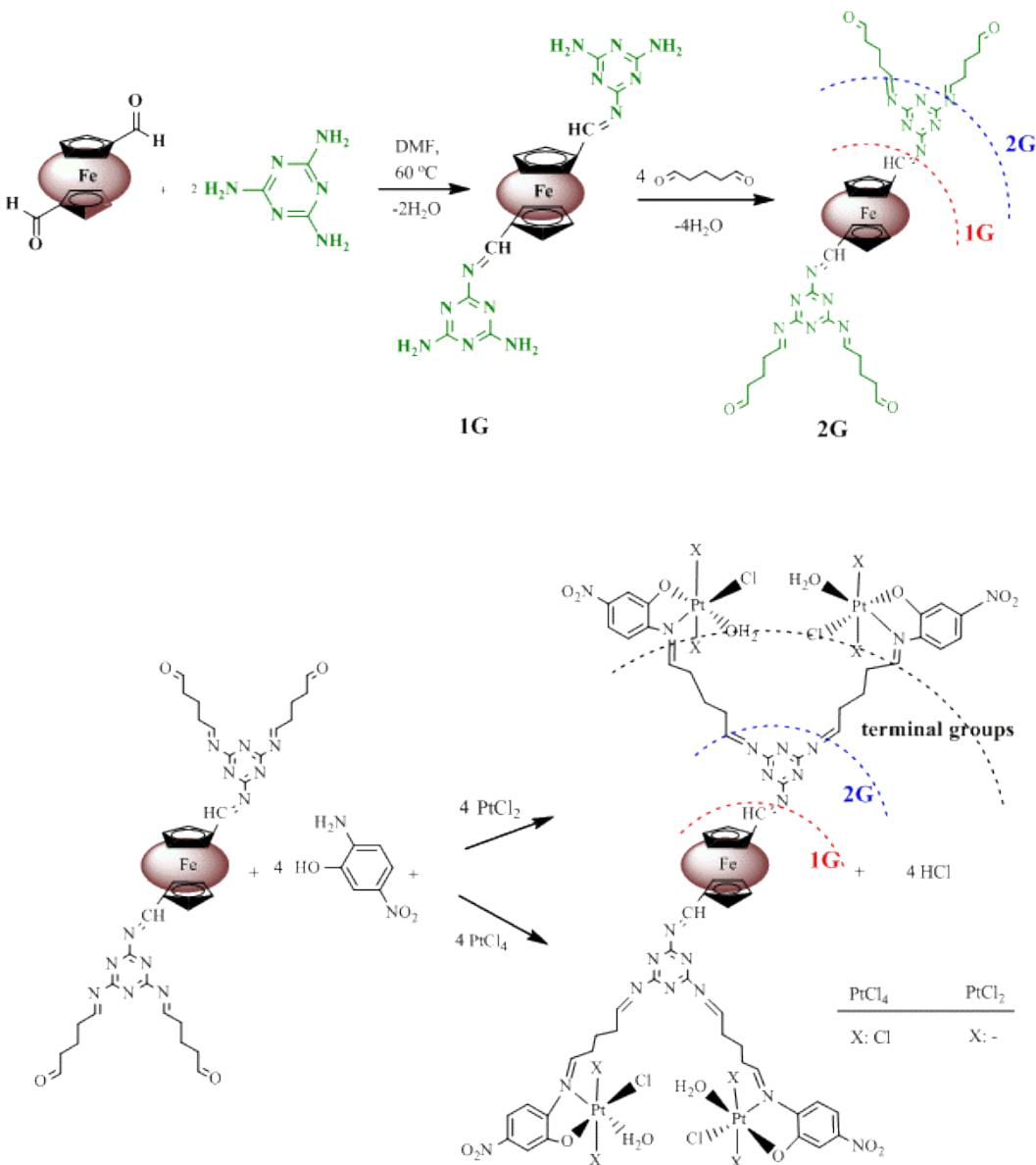
**Fig. 1.** Synthesis schematics of the first, second and extended second-generation dendrimers
