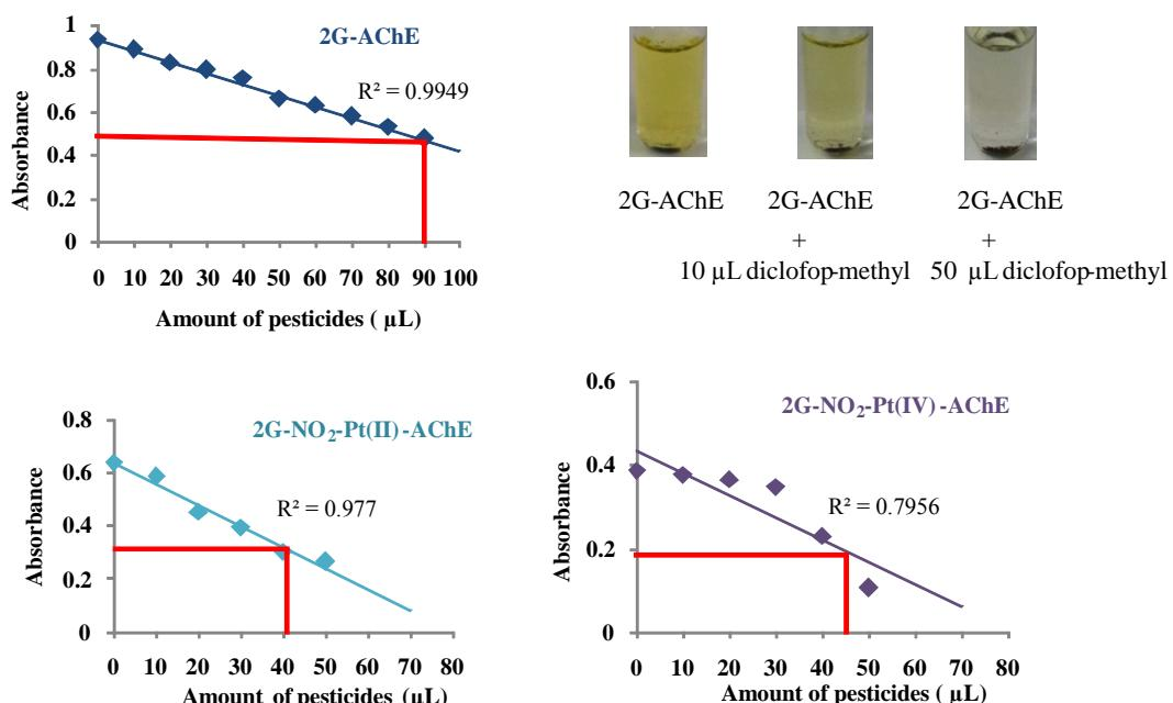
**Fig. 6.** The calibration graphs of the pesticide amounts that are necessary to reduce the enzyme activity by 50 %
