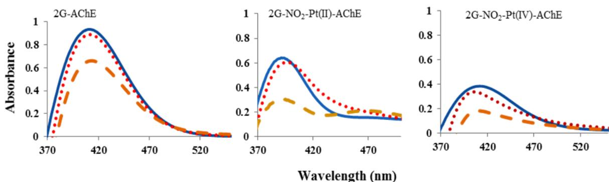
**Fig. 5.** Spectral change of diclofop-methyl herbicide interacting with immobilized dendrimer is given (10  $\mu\text{L}$  diclofop-methyl+immobilized dendrimers (red line); 50  $\mu\text{L}$  diclofop-methyl+immobilized dendrimers (brown line)).
