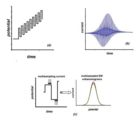
**Fig. 8. (a)** Potential waveform and **(b)** variation of the current with time, considering SWV as a complex repetitive double-step chronoamperometric experiment. **(c)** Current sampling points at different times of each potential pulse and corresponding multi-sampled net SW voltammograms.
