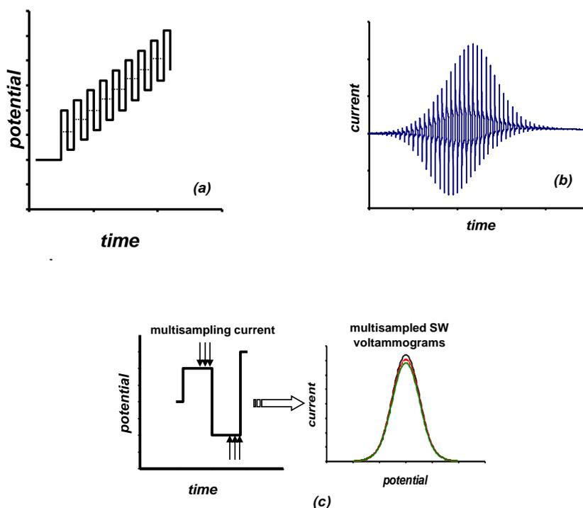
**Fig. 8.** (a) Potential waveform and (b) variation of the current with time, considering SWV as a complex repetitive double-step chronoamperometric experiment. (c) Current sampling points at different times of each potential pulse and corresponding multi-sampled net SW voltammograms.
