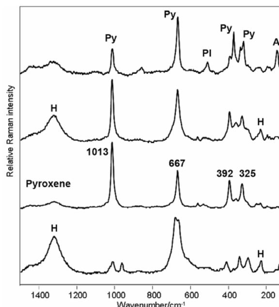
**Fig. 5.** Raman spectra of the mineral pyroxene recorded from recorded from different points on a polished surface of the meteorite *Struga*
