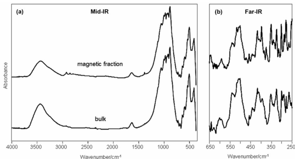
**Fig. 7.** Mid-IR (a) and far-IR (b) spectra of the magnetic fraction (upper spectrum) and of the bulk (lower spectrum) of the meteorite *Struga*
