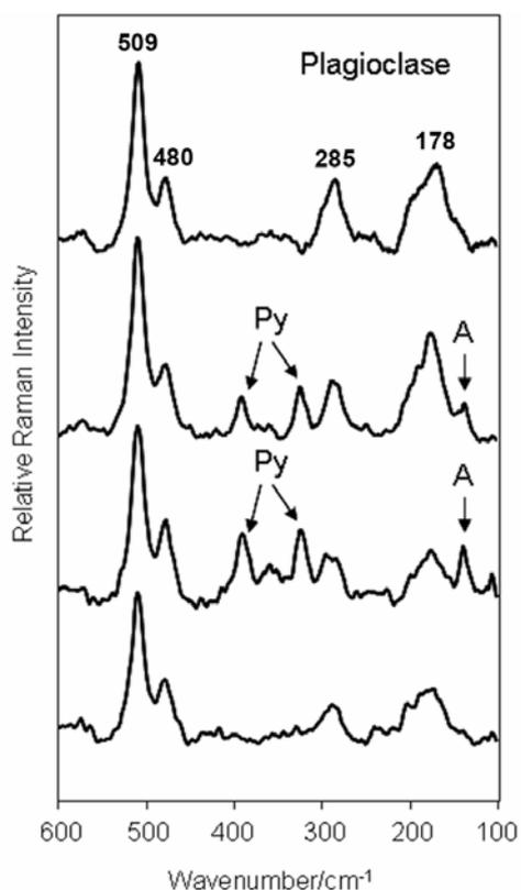
**Fig. 6.** Raman spectra of the mineral plagioclase recorded from recorded from different points on a polished surface of the meteorite *Struga* (A = anatase; Py = pyroxene)
