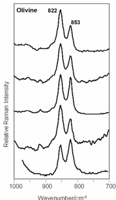
**Fig. 4.** Raman spectra of the mineral olivine recorded from different points on a polished surface of the meteorite *Struga*
