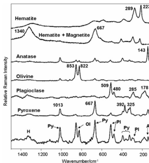
**Fig. 3.** Raman spectra of some minerals recorded from several points on the polished side of meteorite *Struga*. The last spectrum corresponds to the mixture of minerals: A = anatase; Pl = plagioclase; Py = pyroxene; Ol = olivine; H = hematite
