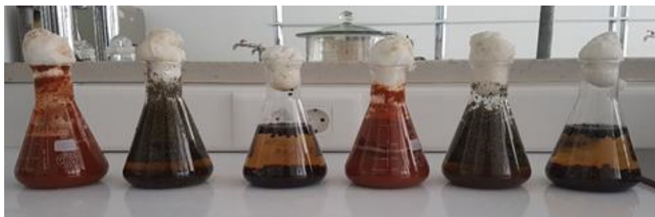
Fig. 1. Extraction of the sample material to be prepared for incubation and enumeration of microbial cells
