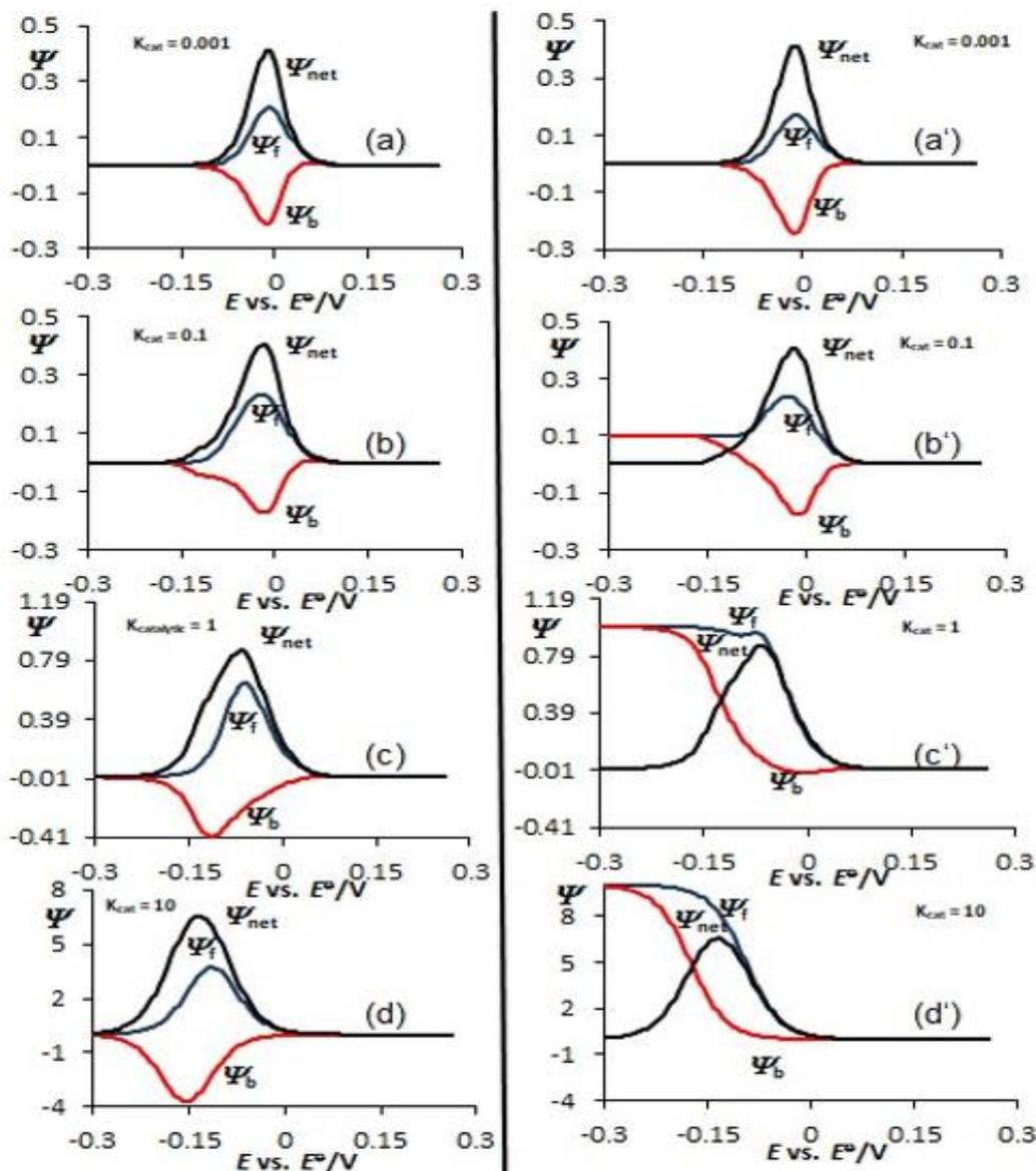
**Fig. 3.** Differential square-wave voltammograms (a–d) and conventional square-wave voltammograms (a'–d') representing the effect of the dimensionless catalytic parameter  $K_{cat}$ . All voltammograms are calculated for the electrode kinetic parameter  $K_{ET} = 0.1$ . For differential square-wave voltammetry (panels a–d) the step-to-pulse duration ratio is  $r = 4$ . The potential increment used was set to  $\Delta E = 4$  mV. Other conditions are same as in Fig. 2.
