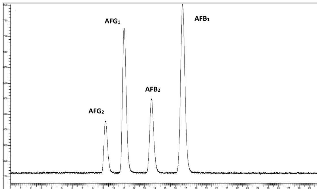
**Fig. 1. (a)** Chromatogram of fortified corn with the concentration of aflatoxins: AFB<sub>1</sub> 5  $\mu\text{g kg}^{-1}$ , AFB<sub>2</sub> 1.55  $\mu\text{g kg}^{-1}$ , AFG<sub>1</sub> 5.12  $\mu\text{g kg}^{-1}$ , AFG<sub>2</sub> 1.46  $\mu\text{g kg}^{-1}$
