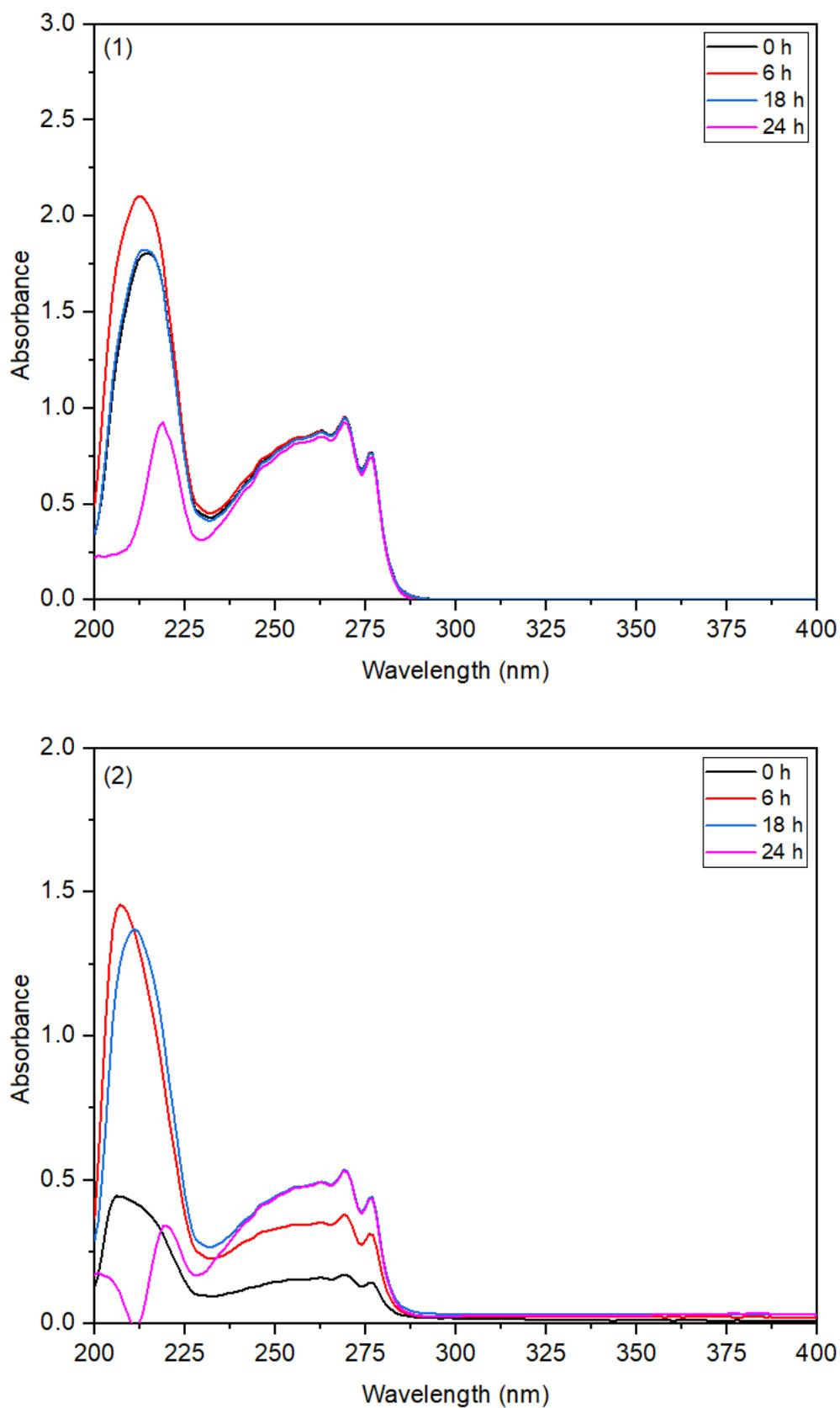
Fig. 5. UV spectra of compounds 1 and 2 in PBS at different time intervals
