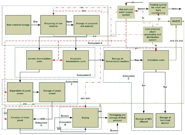
Fig. 1. Block diagram of production system divided to subsystems and "black boxes" (production units) (Colours can be seen on the on line Internet issue)
