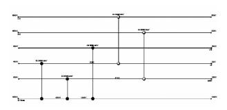
Fig. 8. Grid diagram for new HEN designed with HX-NET (alternative 1/variation 1)
