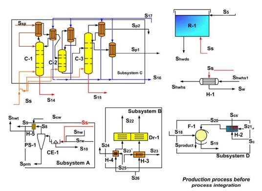
Fig. 2. Flowsheet with selected subsystems of process plant.
