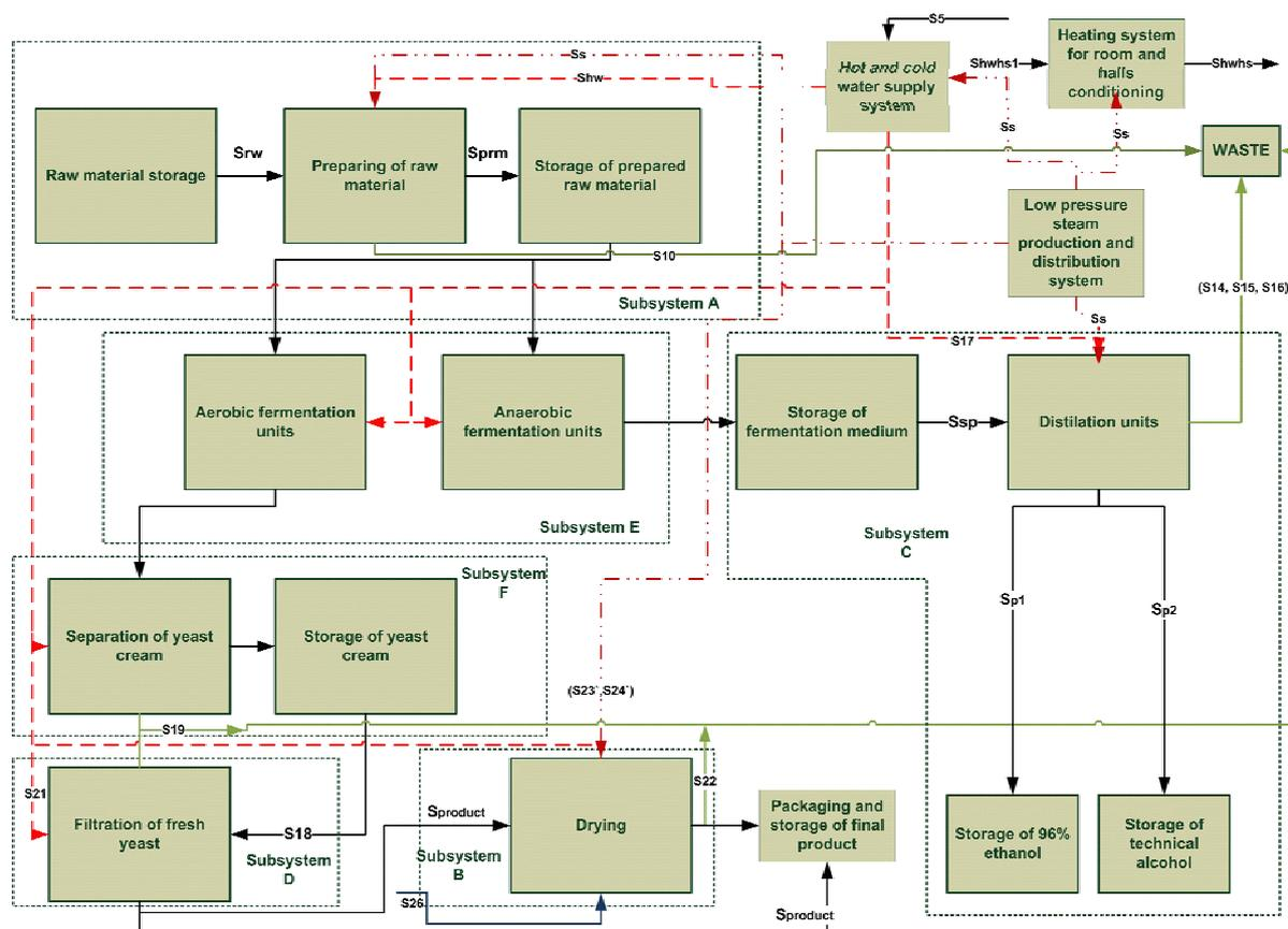
Fig. 1. Block diagram of production system divided to subsystems and “black boxes” (production units) (Colours can be seen on the on line Internet issue)
