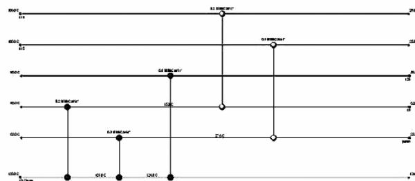
Fig. 8. Grid diagram for new HEN designed with HX-NET (alternative 1 / variation 1)
