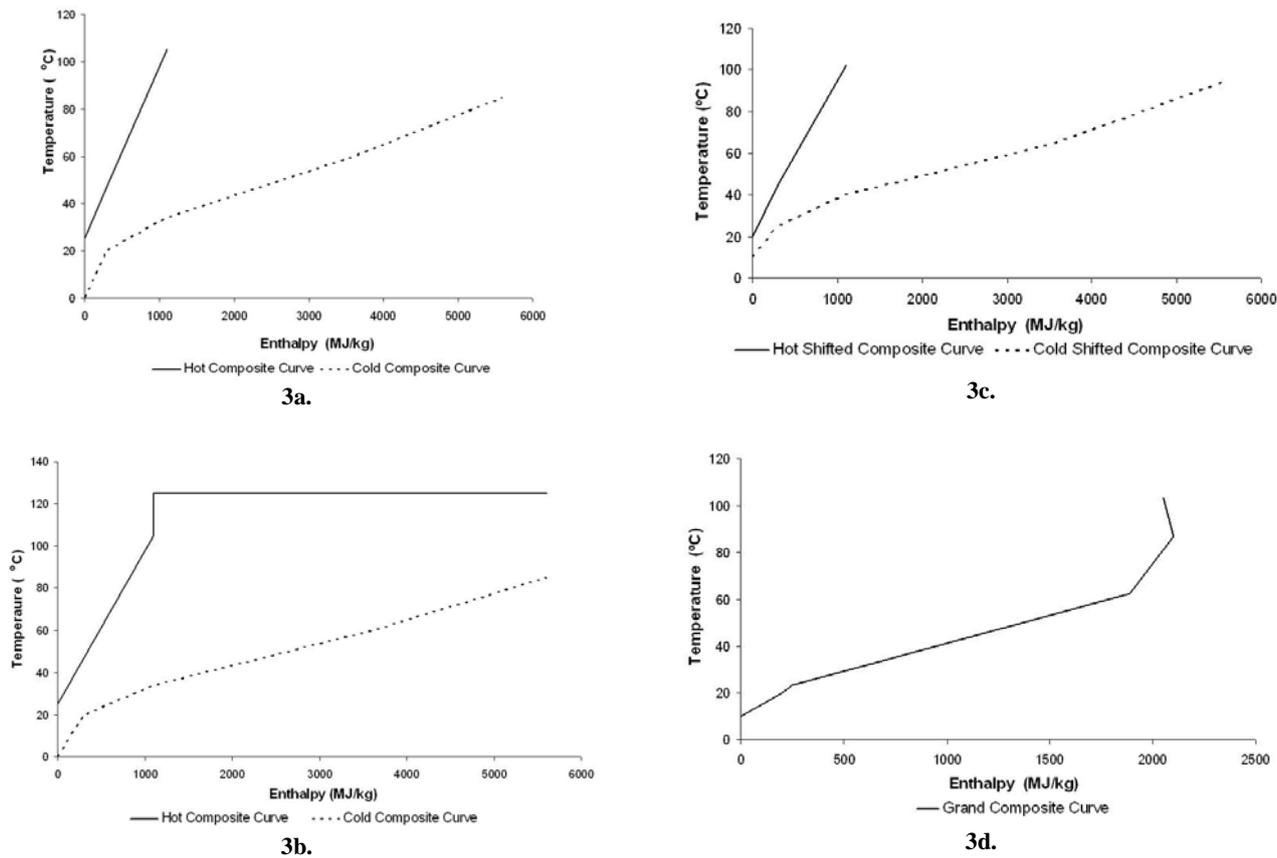
Fig. 3. Composite curves for the system (alternative 1 / variation 1)
