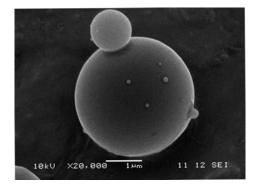
Fig.1. Scanning electron micrograph of TEOS based loaded microparticles
