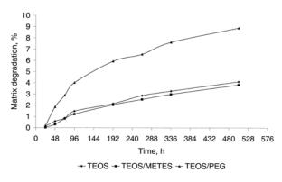
Fig 4. Degradation of different xerogel formulations
