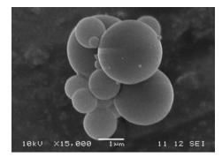
Fig. 2. Scanning electron micrograph of TEOS/ $\alpha$ , $\omega$ -silane-terminated PEG loaded microparticles.
