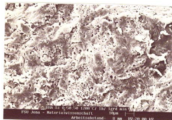
Fig. 4. SEM micrograph of HA : \text{SiO}_2 = 50 : 50\% (bar 10 \mu\text{m} )
