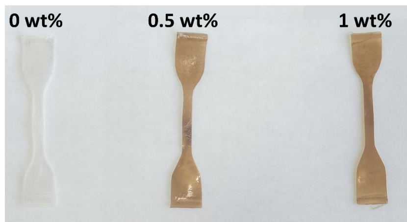
Fig. 1. Free-standing films of the neat polymer (0 wt%) and composites containing 0.5wt% and 1wt% lignin
