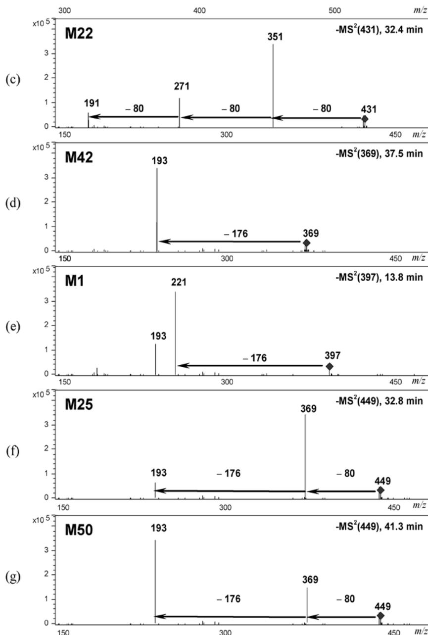
**Fig.4.** MS<sup>2</sup> spectra of some characteristic metabolites of phenolic acids present in urine (c) quinic acid trisulfate (d) ferulic acid glucuronide; (e) dimethylferulic acid glucuronide; (f, g) ferulic acid glucuronide-sulfate
