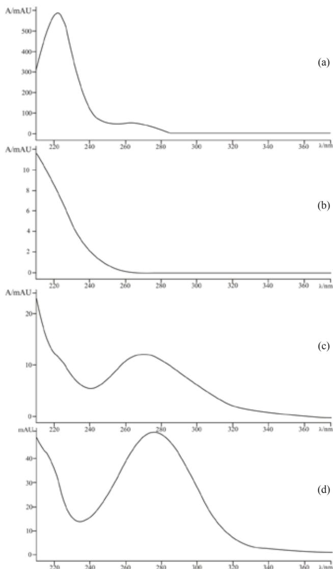
**Fig. 2.** The UV spectra of pure analytical standards of atrazine (a), malathion (b), fenitrothion (c), and parathion (d) in acetonitrile/water (50/50, V/V)
