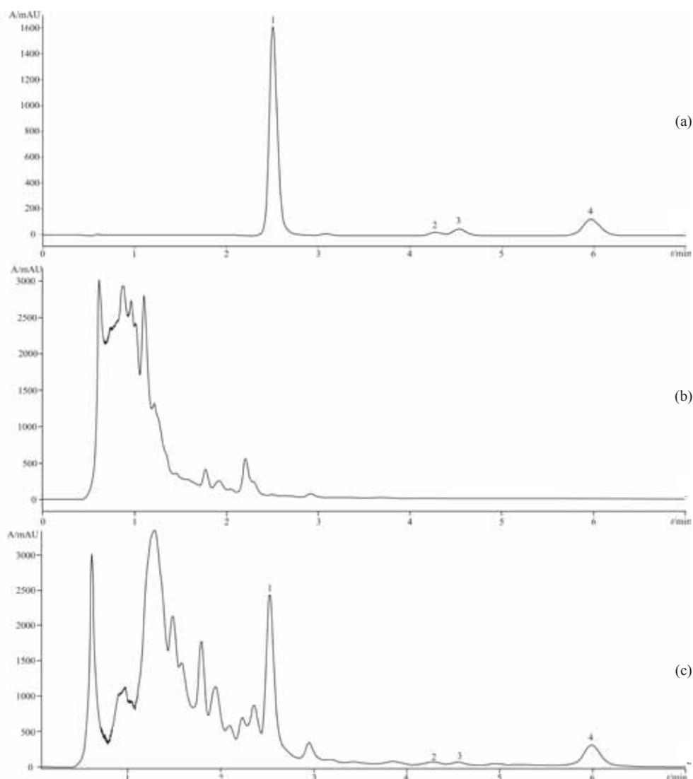
**Fig. 4.** Chromatograms obtained from standard mixtures of atrazine (1), malathion (2), fenitrothion (3), and parathion (4) at the corresponding concentrations to MRLs (a), unspiked apple juice (b), and sample of apple juice fortified at the MRL for each analyte (c) at 220 nm on LiChrospher 60 RP-select B column, with acetonitrile/water (55/45, *V/V*) as the mobile phase
