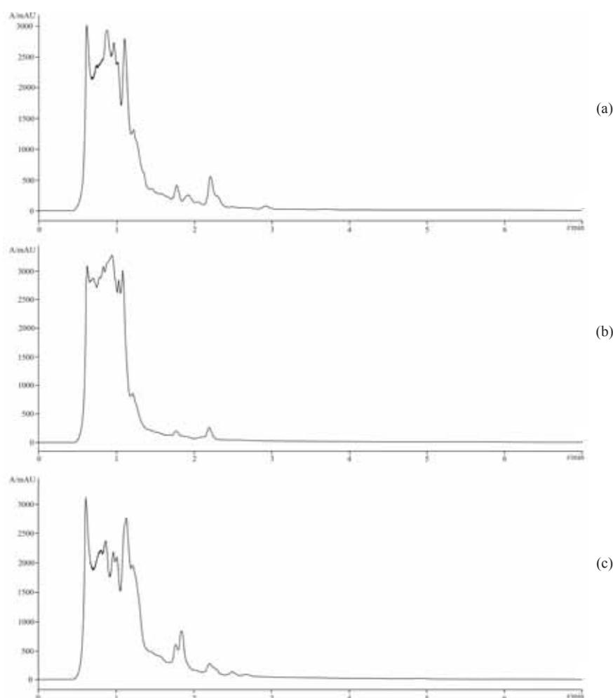
**Fig. 5.** Typical chromatograms of apple juice samples A (a), B (b), and C (c) at 220 nm on LiChrospher 60 RP-select B column, with acetonitrile/water (55/45,  $V/V$ ) as the mobile phase
