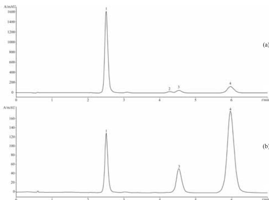
Fig. 3. Chromatograms obtained from standard mixtures of 1  $\mu\text{g}$  atrazine (1), 0.4  $\mu\text{g}$  malathion (2), 0.2  $\mu\text{g}$  fenitrothion (3), and 1  $\mu\text{g}$  parathion (4) at 220 nm (a) and 270 nm (b) on LiChrospher 60 RP-select B column with acetonitrile/water (55/45,  $V/V$ ) as the mobile phase
