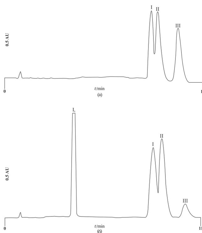
**Fig. 4.** Chromatograms obtained from desmedipham (I), phenmedipham (II) and ethofumesate (III) on the LiChrospher 60 RP-select B column with 60:40 (V/V) methanol-water as mobile phase: (a) standard mixture (1.248  $\mu\text{g}$  desmedipham, 1.296  $\mu\text{g}$  phenmedipham, 6.496  $\mu\text{g}$  ethofumesate); (b) pesticide formulation "Inter OF" (1.548  $\mu\text{g}$  desmedipham, 1.986  $\mu\text{g}$  phenmedipham, 2.491  $\mu\text{g}$  ethofumesate)
