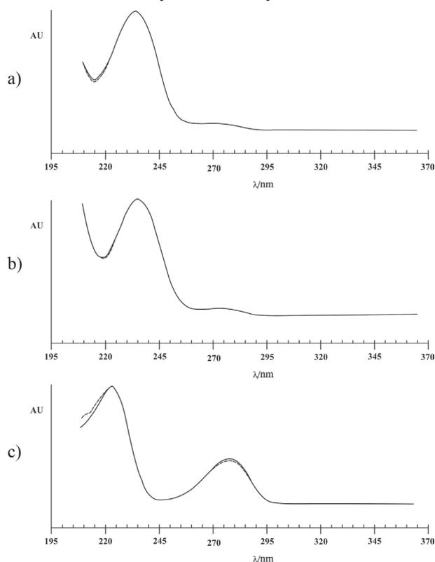
**Fig. 2.** Overlaid UV spectra obtained by comparing the absorption spectra of a pure analytical standard of active ingredient and absorption spectra of the same analyte in the pesticide formulation for (a) desmedipham (1.548 μg), (b) phenmedipham (1.986 μg) and (c) ethofumesate (2.491 μg) in methanol/water (60/40, V/V)
