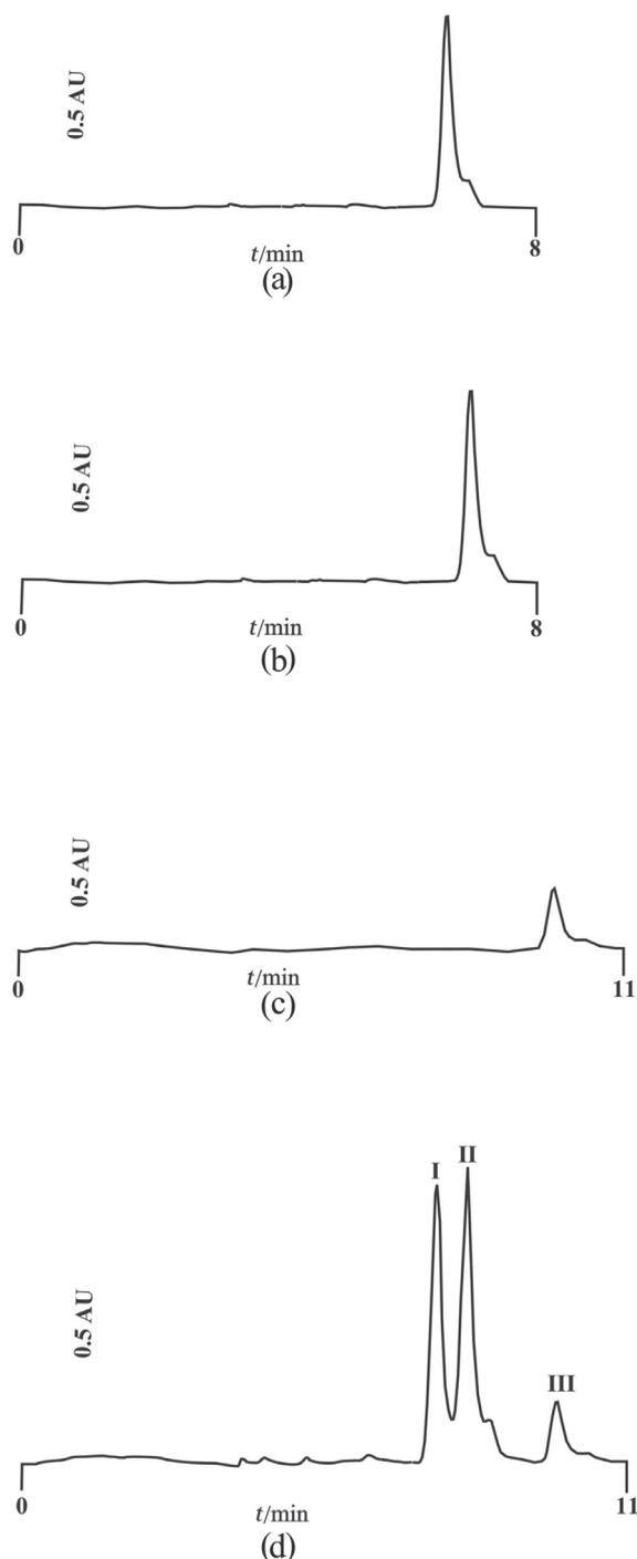
**Fig. 3.** Chromatograms obtained from analytical standard (0.5  $\mu\text{g}$ ) of desmedipham (a), phenmedipham (b) and ethofumesate (c) and their standard mixture (d) on the Hypersil ODS column with 60:40 (V/V) methanol-water as mobile phase
