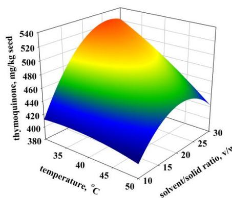
**Fig. 2.** Response surface of thymoquinone content of MAE extract as a function of the temperature and solvent/solid ratio. A time of 25 min was the constant value in the model.
