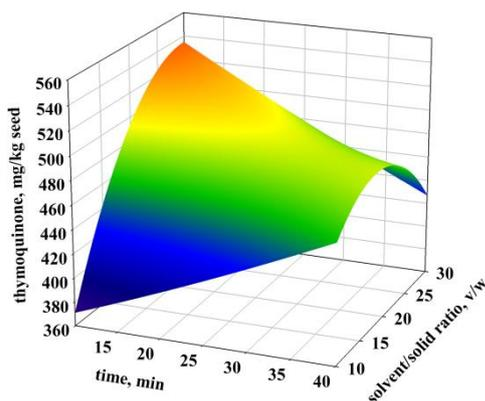
**Fig. 4.** Response surface of thymoquinone content of MAE extract as a function of time and solvent/solid ratio. A temperature of 40 °C was the constant value in the model.
