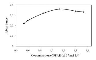
Fig. 2. Effect of SPAR concentration on the extraction of copper. Conditions:  $[Cu] = 26.5 \ \mu g \ l^{-1}$ ,  $[TX-100] = 0.16\% \ (w/v)$ ,  $[Ph]= 0.6\% \ (w/v) \ and \ [pH]= 8.0$
