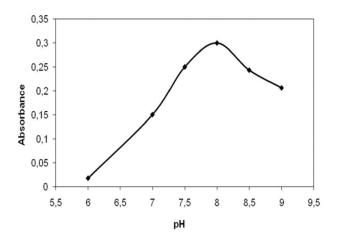
Fig. 1. Influence of pH on the extraction of Cu (II). Conditions: [SPAR] = $1.4 \times 10^{-5}$  mol 1<sup>-1</sup>, [Cu] = $26.5 \ \mu g$  1<sup>-1</sup>, [TX-100] = 0.16% (*w*/*v*) and [Ph] = 0.6% (*w*/*v*).
