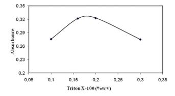
Fig. 3. Variation in the analytical signal of copper as a function of Triton X-100 concentration. Conditions:  $[SPAR] = 1.4 \times 10^{-5} \text{ mol } l^{-1}$ ,  $[Cu] = 26.5 \ \mu g \ l^{-1}$ ,  $[Ph] = 0.6\% \ (w/v) \text{ and } [pH] = 8.0$
