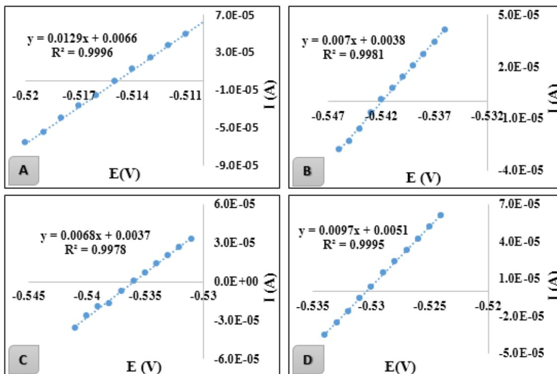
Fig.2. Polarization resistance measurements of Fe electrode in 0.001 M sulfuric acid:
