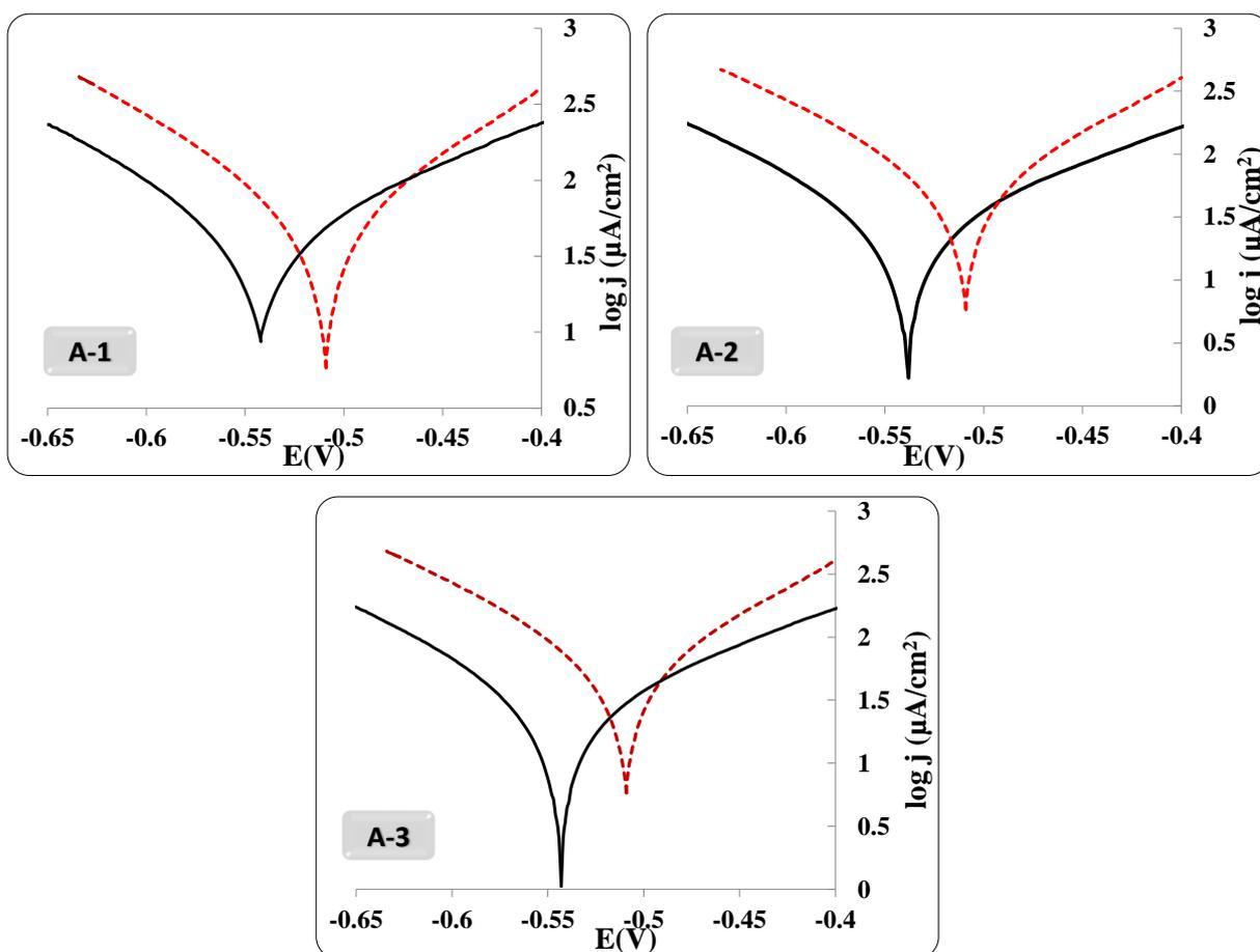
**Fig. 1.** Polarization curve for mild steel in 0.001 M  $H_2SO_4$  in the presence (line) and absence (red dashed line) of: A-1. 4,5-dimethylthiazol-2-amine; A-2. 5-bromothiazol-2-amine; A-3. 5 mM 6-ethoxybenzo[*d*]thiazol-2-amine (red dashed line) at a scan rate of 1 mV/s (measured at 25 °C), and an inhibitor concentration 5 mM.
