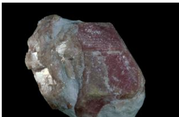
Fig. 2. The corundum crystal of gem quality (6 cm high) is overgrown with diaspore with well visible silvery reflection. Photo: Cyril Mlinar
