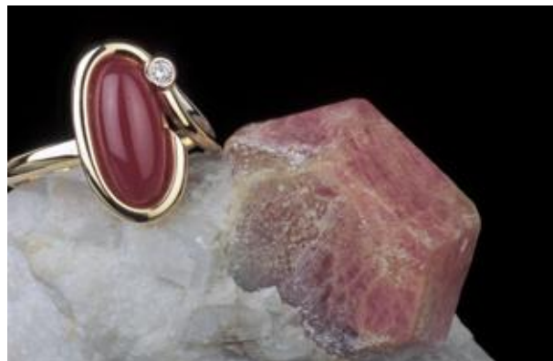
Fig. 5. The basic plane of cabochon of ruby is perpendicular to the direction of parting and that the colour of the ruby was therefore most uniform. Photo: Ciril Mlinar
