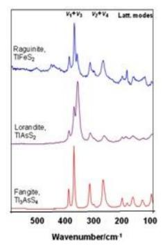
Fig. 20. Raman spectra of some thalium sulfosalts
