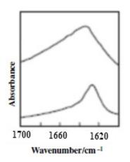
Fig. 13. Cymrite (top) and montmorillonite: the  $\delta$ (HOH) region
