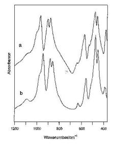
Fig. 6. IR spectra of almandine (a) and spessartine (b)
