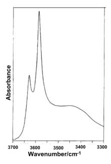
Fig. 11. Carpholite: the O-H stretching region
