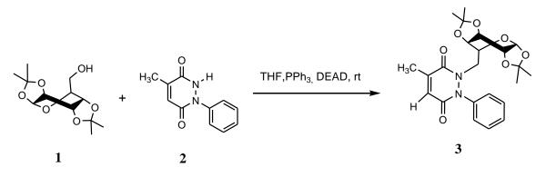
Scheme 1. Substrate scope for the synthesis of glycol-pyradizine-3,6-dione 3
