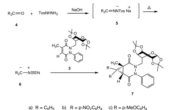
Scheme 2. Proposed synthesis of cyclopropanes using diazo compounds generated in situ
