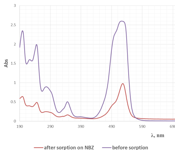
Fig. 5. UV/VIS spectra of Rh6G before and after sorption onto NBZ ( \lambda = 526 \text{ nm} )
